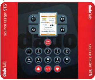
The ST5 Evo can work with all Pitot tubes and thermocouples, it's possible to enter the information related to Pitot tubes in the internal library.
